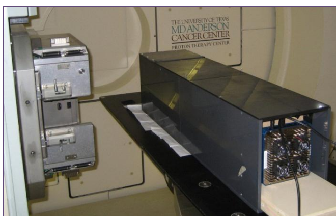
Experimental setup for proton beam measurements with the scintillator detector.
